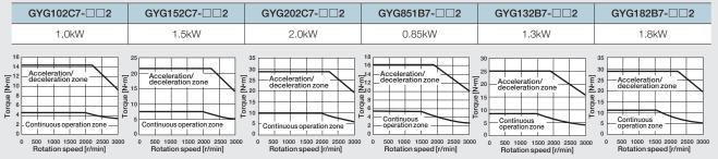
These characteristics indicate typical values of each servomotor combined with the corresponding RYT-7 type servo amplifier.
