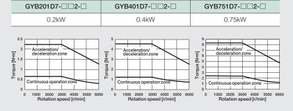
These characteristics indicate typical values of each servomotor combined with the corresponding RYT-7 type servo amplifier. The rated torque indicates the value obtained when the servo amplifier is installed to the following aluminum heat sink.
