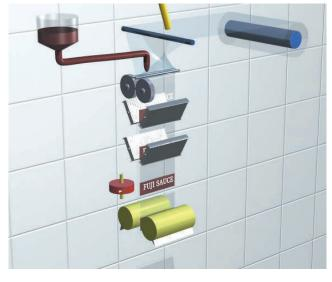
synchronizing the feed, seal, and cut axes Interpolation operation mode and feed forward control Enable interrupt input
